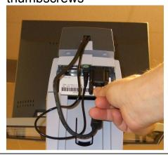
**Step 11:** Connect cord from power supply with the flat side of the plug facing away from the unit
