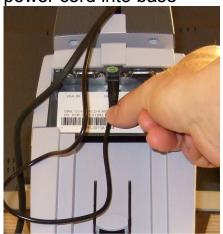
**Step 10:** Connect monitor cable to the base. Tighten thumbscrews
