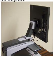
Step 6: Connect monitor cable to the screen. Tighten thumbscrews
