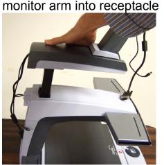
Step 4: Carefully slide monitor onto the monitor arm
