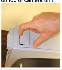
Step 3: Carefully insert monitor arm into receptacle
